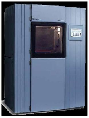
package. The model or part is produced by extruding small beads of thermoplastic material to form layers as the material hardens immediately.
